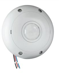
The sensor shall detect occupancy in the control area by detecting Doppler shifts in transmitted ultrasound and passive infrared heat changes. Detection verification of both technologies must occur in order to activate lighting systems. Upon verification, detection by either shall hold lighting on.
