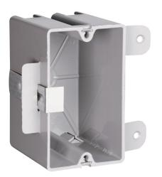
Single-Gang, Wood and Steel Stud Bracket Box. 1/2-inch offset for wood and steel stud mounting. Rear stabilizing bar virtually eliminates inward movement. Two Quick/Click Entries for each end. For use with 3/8-inch to 5/8-inch wallboard. 100 pack.
