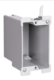
Single gang, deep old work switch and outlet box with Quick/Click and Swing-Bracket for mounting, adjusts from 1 1/4 down to 1/8. It has twoAuto/Clamps foreach end. It has a durable, impact-resistant thermoplastic box. The metal swing bracket is for quick mounting in existing walls. 50 pack.
