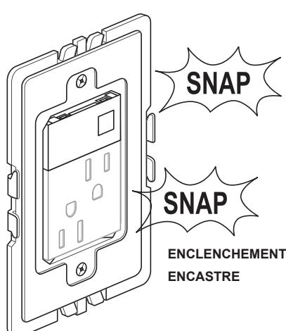
**NOTE** - If you need to remove night light after snapping into frame, first remove frame from wall box to access the two locking tabs on the back of the night light. Insert a flat screwdriver to depress tabs as you apply pressure to push night light out.
