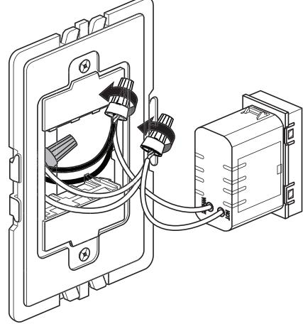
If you have 4 wires plus a ground, use wire nut to connect both HOT wires together with HOT wire from night light. Connect both WHITE wires together with WHITE wire from night light. To maintain existing wire circuit, a jumper wire must be added for second device (outlet).
