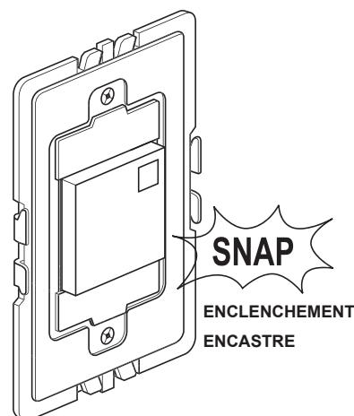
**NOTE** – If you need to remove night light after snapping into frame, first remove frame from wall box to access the three locking tabs on the back of the night light. Insert a flat screwdriver to depress tabs as you apply pressure to push night light out.
