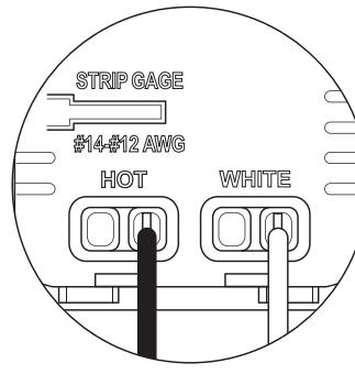
**WARNING:** Do not pair different size wires in the same terminal. If you have different size wires, use a wire nut to add a 6 inch pigtail of the same gauge wire to the smaller gauge wire.
