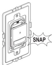
**NOTE – If you need to remove sensor after snapping into frame, first remove frame from wall box to access the four locking tabs on the back of the sensor. Insert a flat screwdriver to depress tabs as you apply pressure to push switch out.**
