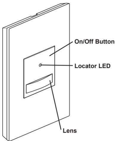
The ASVS12 is designed to replace a standard single pole or multi-way light or fan switch. The sensor uses passive infrared technology to sense human motion in a space and turn the lights or fan OFF when the room is vacant. It is ideal for applications in a home where there is a direct line of sight from the sensor to the room such as bedrooms and family/living rooms.
