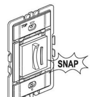
NOTE – If you need to remove a device from the frame, remove frame from wall box. Insert a flat screwdriver from the back of the frame and depress the tabs on the device to unlock and push it forward.
