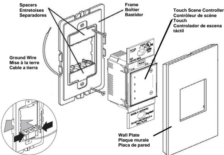
Remove spacers from the frame. Since this device fills the frame completely, you will not need the spacers. From the back of the frame, pinch the tabs on the spacer to release.
