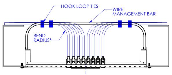
\* THE MINIMUM CABLE BEND RADIUS IS 4 TIMES THE OUTSIDE CABLE DIAMETER. HOOK LOOP TIE WRAPS SHOULD BE USED TO ATTACH THE CABLES TO THE WIRE MANAGEMENT BAR. THE CABLE AT THE EDGE OF THE PATCH PANEL SHOULD BE ATTACHED TO THE CABLE WHICH HAS ALREADY BEEN TIE WRAPPED TO THE WIRE MANAGEMENT BAR.
