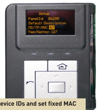
The easiest way to change Device IDs and set fixed MAC addresses on network bridges is to follow the prompts on an LMCT-100. Set LILM panel addresses with each panel's built-in user interface.
