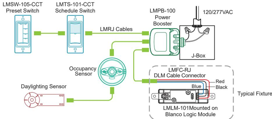
NOTE: Each DLM local network must include a DLM room controller, relay panel, or power booster to supply low voltage power to the LMLM-101.
