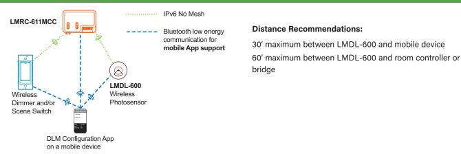
**NOTE:** LMDL-600 must be connected to an LMRC-611 series room controller. It cannot communicate with the LMBC-650 wireless bridge.
