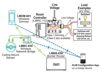
Note: For a single (non-networked) hybrid room, the LMBR-650 is not required.
