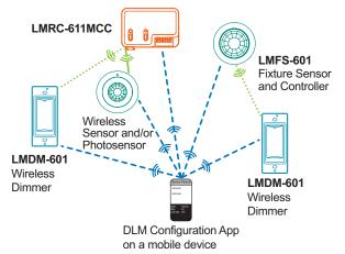
(Note that a single LMDM-601 can control both wireless room controllers and the LMFS-601.)
