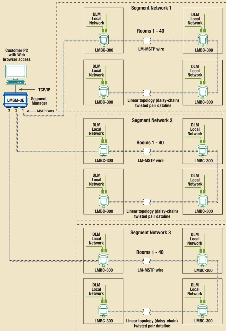
Figure 2. Basic system with 3 segment networks
