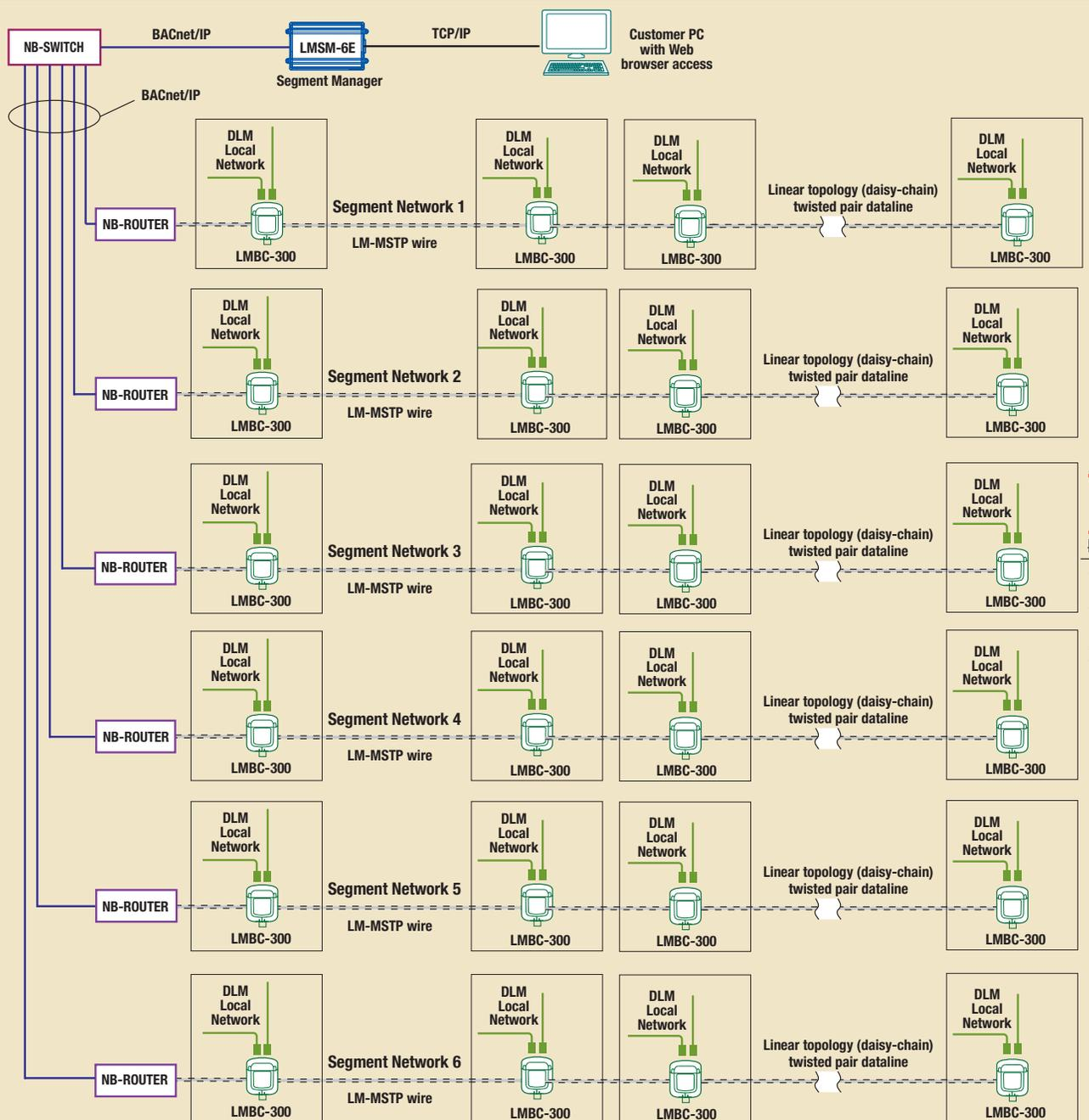
Figure 3. Advanced system with 6 segment networks. See CAD Resource drawings 90-775, 90-775-1 and 90-776 for additional information.
