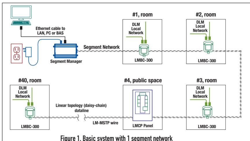
Figure 1. Basic system with 1 segment network
