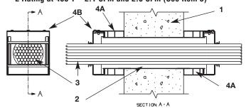
Wall Assembly – Min 4-1/2 in. [114 mm] thick reinforced lightweight or normal weight (100-150 pcf or 1600-2400 kg/m3) concrete for 1 and 2 hr rated assemblies. Min 6 in. [152 mm] thick reinforced lightweight or normal weight (100-150 pcf or 1600-2400 kg/m3) concrete for 3 and 4 hr rated assemblies. Wall may also be constructed of any UL Classified Concrete Blocks. Diam of opening shall be 2-1/4 in. [57 mm] or 4-3/4 in. [121 mm] for the nom 2 in. [51 mm] and 4 in. [102 mm] sleeves (Item 2).
