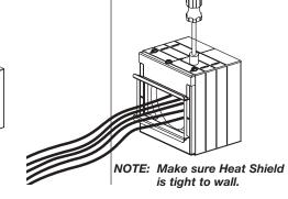
**5.** Move Sliding Doors to be snug around Cables by turning Side Screws.
