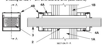
Wall Assembly – The 1, 2, 3 or 4 hr fire-rated gypsum board/stud wall assembly shall be constructed of the materials and in the manner described within the individual U300, U400 or V400 Series Wall or Partition Designs in the UL Fire Resistance Directory and shall incorporate the following construction features:
