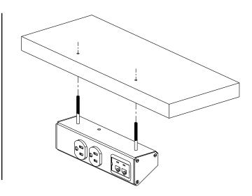
NOTE: Use No. 10-32 nut and washer to secure mounting studs into mating holes in mounting surface.
