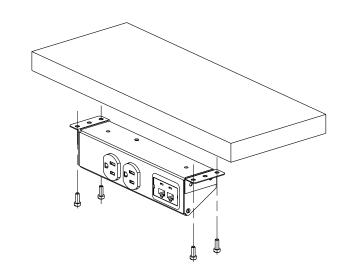
NOTE: Use No. 8 (5/16" [7.9mm] head size) round head fastener or equivalent to secure mounting flange onto mounting surface.
