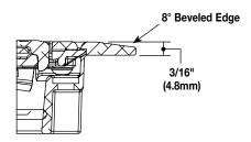
NOTE: All surface style poke-thru devices come with a transition angle to aid in the change in floor elevation.
