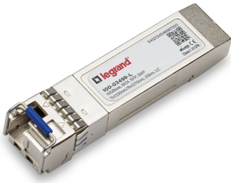
Calix 100-03499 Compatible 10GBase-BX SFP+ Transceiver (SMF, Tx: 1330nm Rx: 1270nm, 10-20km, LC Duplex, DDM, I-Temp)
