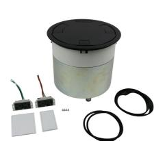
For use with 10" (254mm) diameter hole. Cover and stem are pre-assembled together. All devices are recessed 4 1/2" (114mm) below the finished floor level. Unit ships complete with an all aluminum cover (assembled) designed to sit on top of finished floor surface (carpet, tile, wood, concrete or terrazzo). Covers are available in the following powder coated finishes: black (BK), gray (GY), nickel (NK), brass (BS) and aluminum (AL).
