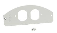
Single-gang device plate that accepts standard 20A duplex receptacle or a duplex Turnlok receptacle. Fits in any one (1) of the shaded locations shown. Devices supplied by others.
