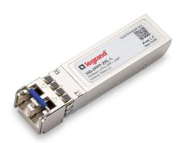
Brocade 10G-SFPP-ZRL Compatible 10GBase-LR70 SFP+ Transceiver (SMF, 1310nm, 70km, LC Duplex, DDM, C-Temp)
