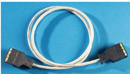
Clarity® 110 patch cords are ETL verified to Category 6 and 5e component standards. Clarity 110 plugs utilize an internal signal feedback technique to control cross talk without compromising impedance.
