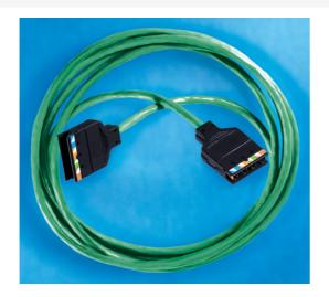
Clarity 110 patch cords are ETL verified to TIA-568-B Category 6 and 5e component standards. More importantly, Clarity 110 plugs utilize an internal signal feedback technique to control cross talk without compromising impedance. Clarity 110 to modular 8 position patch cords utilize both signal feedback and center tuning. This allows more transparent connector interfaces for significant elevation of channel performance that can be field measured.
