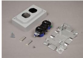
Cover has twistouts for 1500 and 2600 Series Raceway on all four sides. Base has 1/2'' and 3/4'' trade size concentric KOs. Two 1500WC Wire Clips included. Gray finish.
