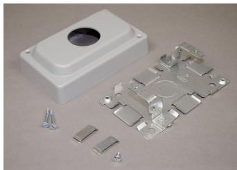
Will accommodate commercially available straight blade and locking single receptacles with face diameters of 1.38-1.40" (35-36mm). Base has 1/2" and 3/4" trade size concentric KOs. Nonmetallic cover has 1500 and 2600 Series Raceway twistouts on all four sides. Two 1500WC Wire Clips included. Gray finish. NOTE: Certified to Canadian Safety Standards. For sale in Canada. When ordering these products, add "C" prefix to part number to denote the Canadian version, i.e "C1546A".
