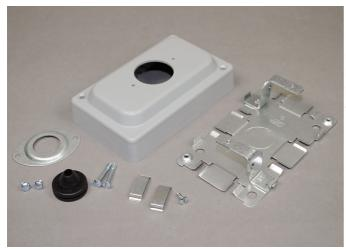
Furnished with 1/2" (12.7mm) rubber stem. Designed to accept modular connecting blocks within the fitting. Nonmetallic cover has 1500 and 2600 Series Raceway twistouts on both ends and both sides. Two 1500WC Wire Clips included. Not UL Listed. Gray finish.
