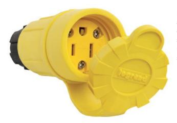
Rated watertight for 1,500 psi high-pressure hosedown, Pass and Seymour plugs and connectors feature multiple seals to ensure protection against the environment. Constructed of a sturdy rubber body, which makes them impact- and chemicalresistant, they have nickel-plated blades and contacts for superior corrosion resistance.
