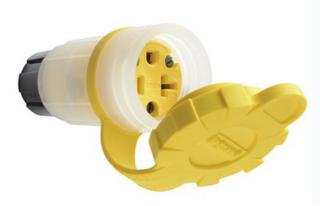
Rated watertight for 1,500 psi high-pressure hosedown, Pass and Seymour watertight GCM plugs and connectors feature multiple seals to ensure protection against the environment. The transparent body houses dual LED lights with 360 visibility, indicating ground continuity and power status, while providing a NEMA 6P/IP67 rating.
