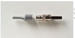
Legrand quick-cure, anaerobic epoxy field-installable connectors speed installation time. Strip the fiber, inject the adhesive into the connector, insert and scribe the fiber, then polish the connector end face to perfection for a high performance termination.
