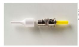
Legrand quick-cure, anaerobic epoxy field-installable connectors speed installation time. Strip the fiber, inject the adhesive into the connector, insert and scribe the fiber, then polish the connector end face to perfection for a high performance termination.
