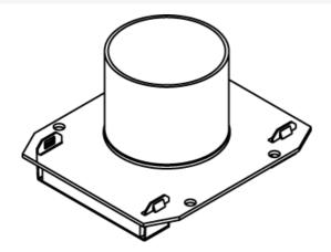
Two-gang 2" trade size conduit housing assembly. Used on 8AT Series devices. Covers two (2) of the three (3) gangs in the center compartment. Only for use with 8AT Series units.
