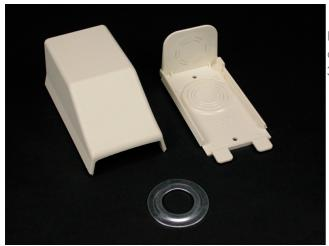
For connecting 2300 Raceway with 1/2", 3/4", or 1" trade size conduit or armored cable. 1/2" and 3/4" trade size KO on end, 1/2", 3/4" and 1" trade size KOs on bottom.
