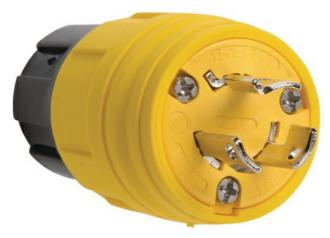
Locking Watertight Plug, 15amp 250volt, NEMA Configuration L6-15, multipoint sealing system provides environmental protection of: NEMA 4, 4X, 6, 6P and IP67 rated.
