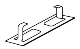
Enables mounting of a duplex receptacle to 25DTP and AMDTP Series Tele-Power Poles.
