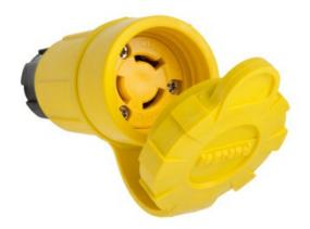
Locking Watertight Connector, 15amp 125volt, NEMA Configuration L6-15, multipoint sealing system provides environmental protection of NEMA 4, 4X, 6, 6P, and IP67 rated.
