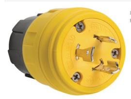
Locking Watertight Plug, 20amp 125volt, NEMA Configuration L5-20, multipoint sealing system provides environmental protection of: NEMA 4, 4X, 6, 6P and IP67 rated.
