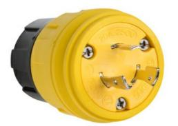
Locking Watertight Plug, 20 amp 250 volt, NEMA Configuration L6-20, multipoint sealing system provides environmental protection of: NEMA 4, 4X, 6, 6P and IP67 rated.
