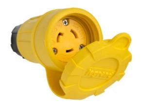
Locking Watertight Connector, 20 amp 250 volt, NEMA Configuration L6-20, multipoint sealing system provides environmental protection of NEMA 4, 4X, 6, 6P, and IP67 rated.
