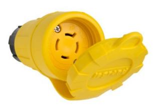
Locking Watertight Connector, 20amp 125/250volt, NEMA Configuration L14-20, multipoint sealing system provides environmental protection of NEMA 4, 4X, 6, 6P, and IP67 rated.
