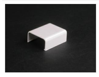
Makes right angle turns around internal corners of 2800 Series Raceway. Maintains 1 1/4'' (32mm) bend radius when installing UTP and fiber optic cable.
