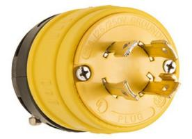
Locking Dust-Tight Rubber Plug, 30amp 125/250volt, NEMA Configuration L14-30
