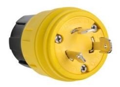
Locking Watertight Non-Grounding Plug, 30amp 125/250volt, multipoint sealing system provides environmental protection of: NEMA 4, 4X, 6, 6P and IP67 rated.
