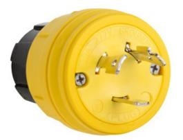
Locking Watertight Plug, 30amp 277volt, NEMA Configuration L7-30, multipoint sealing system provides environmental protection of: NEMA 4, 4X, 6, 6P and IP67 rated.
