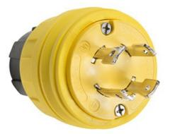
Locking Watertight Plug, 30amp 125/250volt, NEMA Configuration L14-30, multipoint sealing system provides environmental protection of: NEMA 4, 4X, 6, 6P and IP67 rated.
