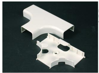
For branching of 2900 Series Raceway running at right angles. Maintains 1 1/4'' (32mm) bend radius when installing UTP and fiber optic cable.
