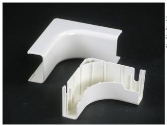
2900 Series Radiused Interior Elbow. Makes right angle turns around internal corners of 2900 Series Raceway running at right angles. Maintains 1 1/4'' (32mm) bend radius when installing UTP and fiber optic cable.
