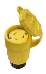
Locking Watertight Connector, 30amp 125volt, NEMA Configuration L5-30, multipoint sealing system provides environmental protection of NEMA 4, 4X, 6, 6P, and IP67 rated.
