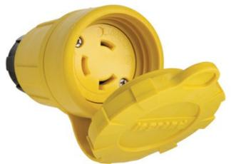
Locking Watertight Connector, 30amp 277volt, NEMA Configuration L7-30, multipoint sealing system provides environmental protection of NEMA 4, 4X, 6, 6P, and IP67 rated.
