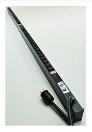
Two circuits with two 15A resettable circuit breakers. Thirty-six 20A outlets with T-slots, black housing. 12' (3.6m) cord. Length 70'' (1.8m).
