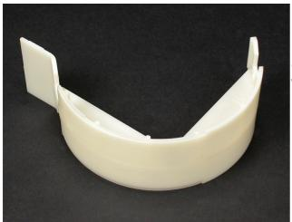
Radiused insert for the 4011 Flat Elbow and the 4015 Undivided Tee. Provides 2" (51mm) cable bend radius control for UTP, STP or fiber optic cable installations. Ideal for new and retrofit applications whether the cable installation is lay-in or pull-through.
